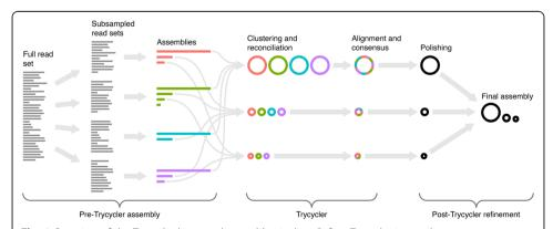
**Fig. 1** Overview of the Trycycler long-read assembly pipeline. Before Trycycler is run, the user must generate multiple complete assemblies of the same genome, e.g., by assembling different subsets of the original long-read set. Trycycler then clusters contigs from different assemblies and produces a consensus contig for each cluster. These consensus contigs can then be polished (e.g., with Medaka) and combined into a final high-quality long-read-only assembly
